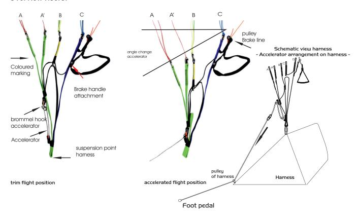
By operating the foot accelerator the pilot shortens the A/B belts by a pulley system which reduces the force.
