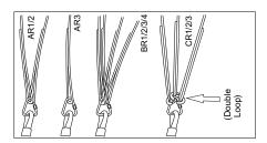
Factory configuration with double loop on Br4 and CR lines for trimming during ageing
