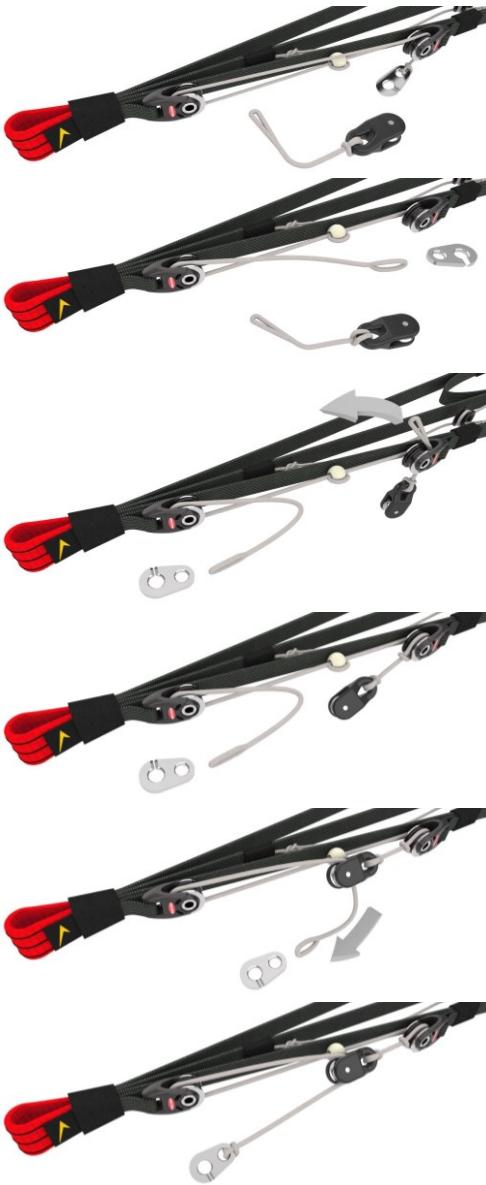
Fig. 9 Installing the speedlimiter
