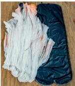
Gather your glider and lay it next to the SOFTBAG. The lines should protrude out of the trailing edge. At the bottom of the SOFTBAG there is a riser bag. here the risers will be stowed away later. The trailing edge should be in the direction of the riser bag.
